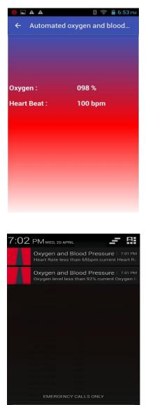
This is a system which measures blood pressure and oxygen level simultaneously in the automated system using embedded system. The output of the system is received on the smartphones via bluetooth, on the screen we will be able to see the high and low bood pressure readings and also the oxygen level in the human body This system is combination of software and hardware. The method we have used is a non-invasive method of measuring the bood pressure and the oxygen level.
